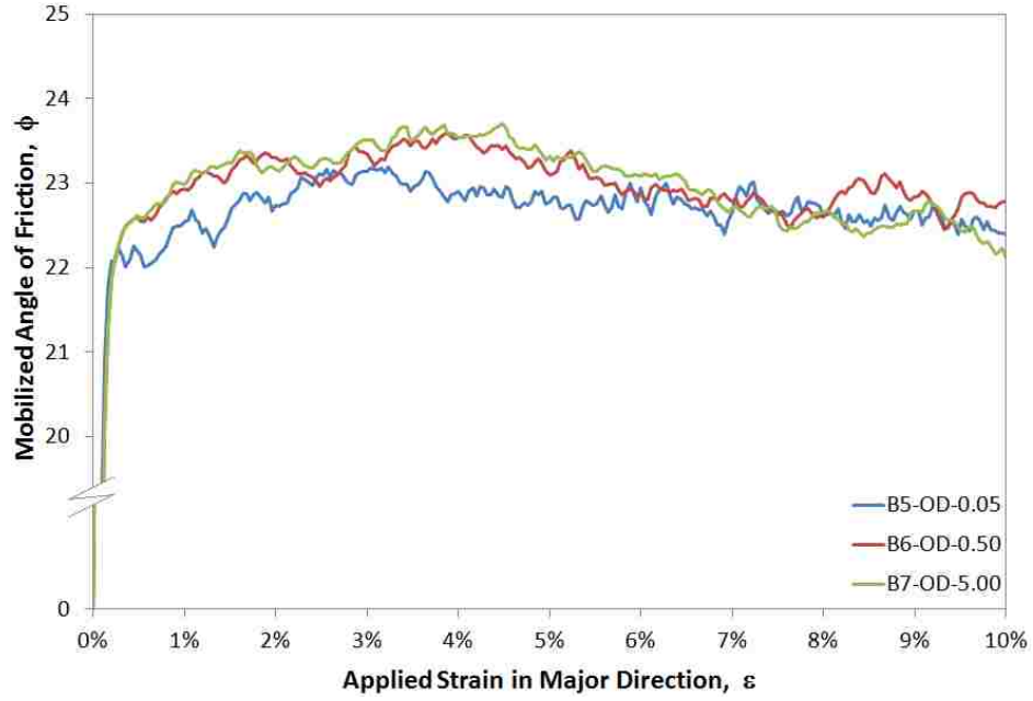
Fig. 55 Friction angle of models with equal \xi \varepsilon' values evolved with applied strain. Blue indicates the model with \xi < \xi_{opt} ; red and green indicate the models with \xi > \xi_{opt} .
